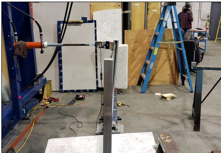
Figure 4. 4 ft. Vista Frameless Glass Railing System Horizontal – Top of Post Concentrated Load
