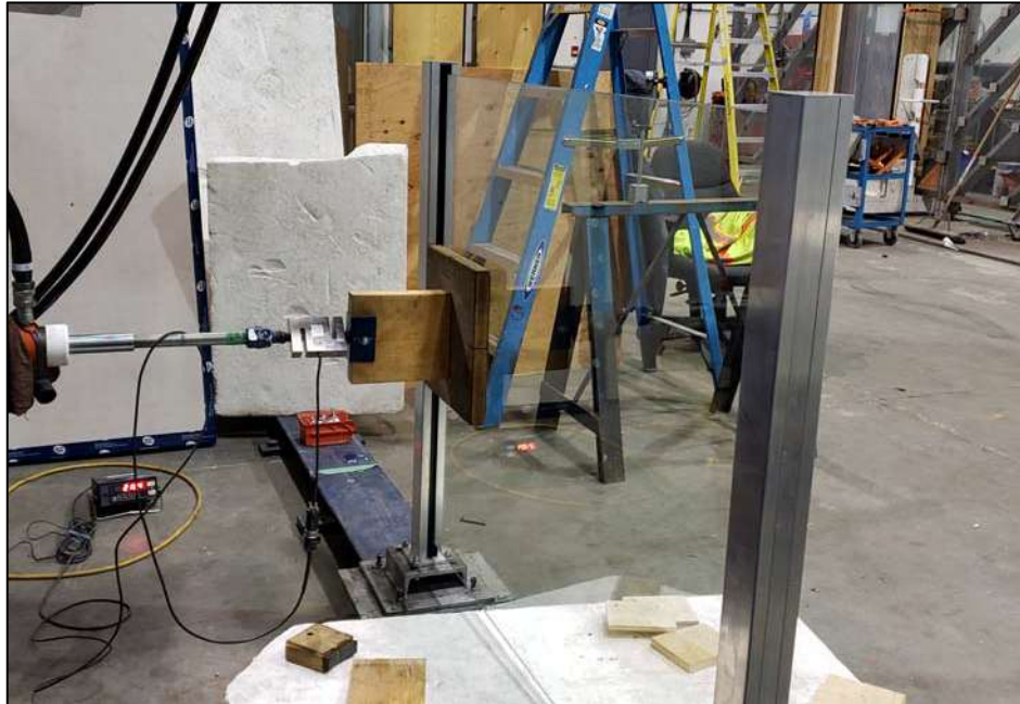
Figure 1. 4 ft. Vista Frameless Glass Railing System – In-Fill Load Test
