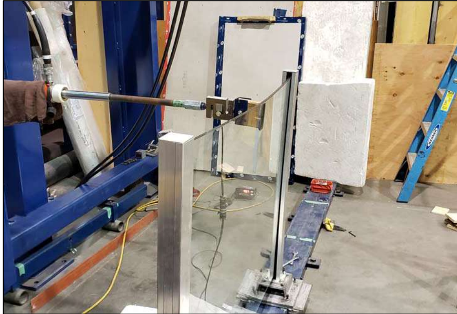
Figure 3. 4 ft. Vista Frameless Glass Railing System Horizontal – Mid-Span of Top Rail Concentrated Load
