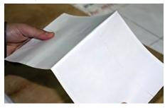
**A-4. Set Corner Fold Width.** Place index finger on the top side of the FlexWrap™ NF at the intersection of CREASE A and CREASE B.
