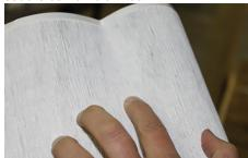
**A-5. Create Corner Fold.** On the reverse side of the FlexWrap<sup>™</sup> NF, starting at the intersection of CREASE A and CREASE B, fold along CREASE B going out towards edge of narrow release paper.
