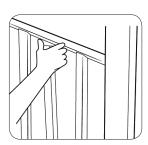
Angle balusters away from you. Starting on one end, insert balusters into top rail. Slide rail into position. Screw brackets to post. Pre-drill holes with 5/32" drill bit.
