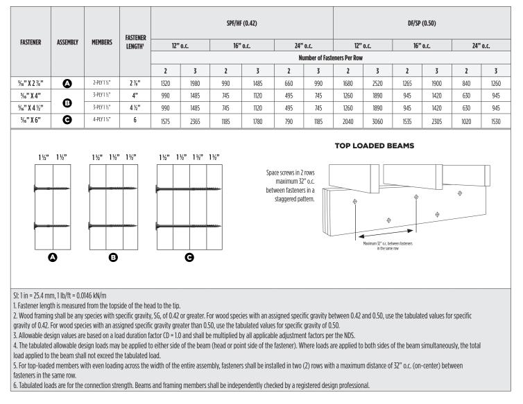
TABLE 1: Allowable Lateral Design Values (plf) for Multi-Ply Truss and Sawn Lumber Assemblies <sup>2,3,4,5,6</sup>
