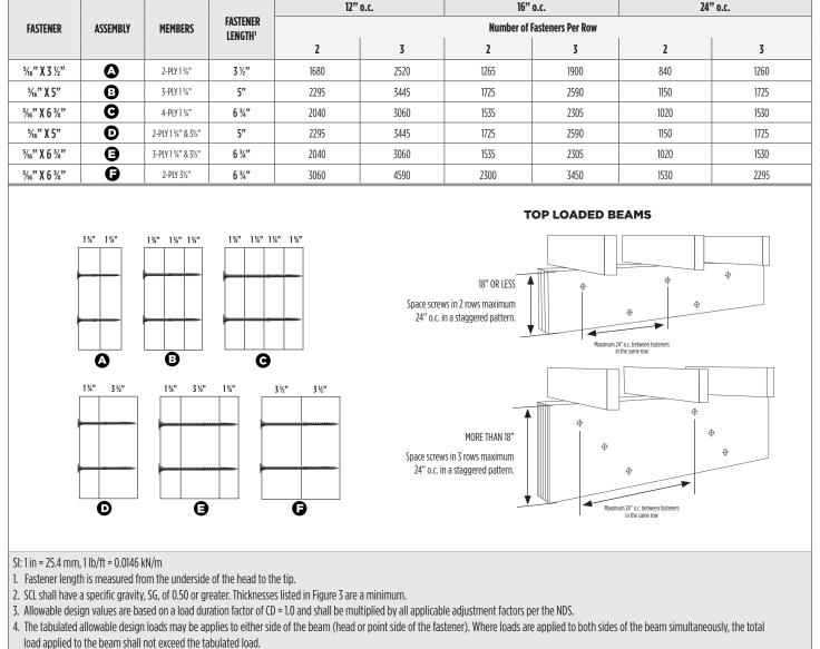
5. For top-loaded members with even loading across the width of the entire assembly, and a depth of 18" or less, fasteners shall be installed in two (2) rows with a maximum distance of 24" o.c. between fasteners in the same row. Use three (3) rows for members deeper than 18".
