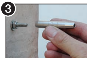
3 Tighten nut to set the anchor. Apply a high strength thread locking compound to threads. Spin Quick-Connect® fitting onto Expansion Bolt until it bottoms out.
