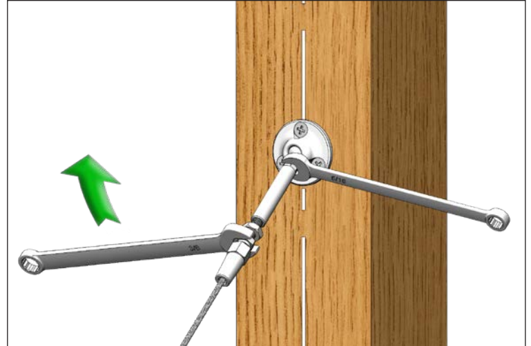
Figure Y. Hold the tensioner terminal still with a 3/16" wrench and using a 5/16" open wrench, rotate tensioner body to tension.
