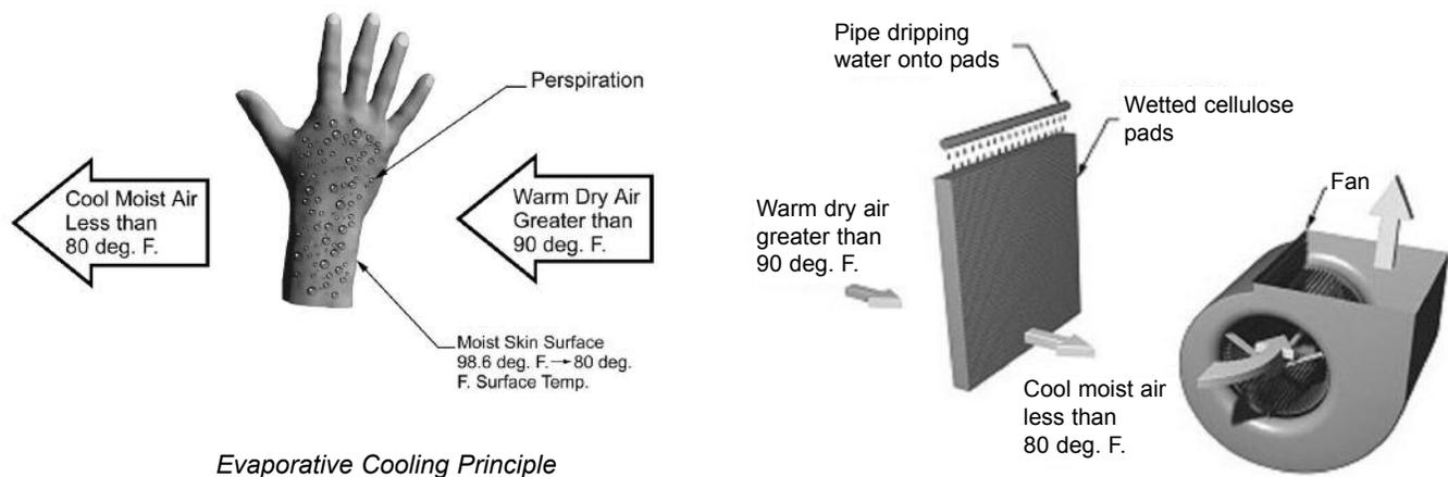
Evaporative cooling is the same process your body uses to cool itself. When you perspire, and air moves across your skin, a portion of the perspiration (water) evaporates. Evaporation requires heat to change liquid water to water vapor and this heat is taken from your skin, producing the cooling effect.
