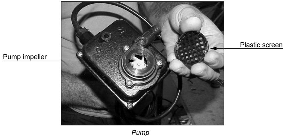
A small plastic screen covers the pump inlet to prevent foreign matter from entering and damaging the pump impeller. The screen snaps in place and can be easily removed for inspection or cleaning.
