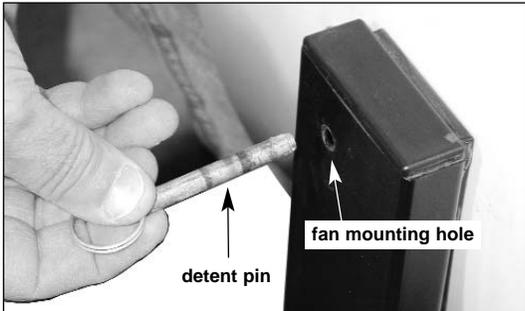
Insert a detent pin through the left side of the fan mounting hole in the upright into the hole in the left side of the fan. Repeat this step for the right side.
