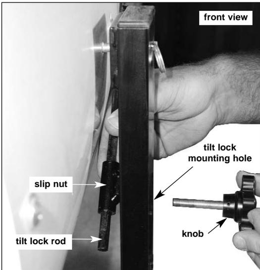
Insert the knob through the tilt lock mounting hole in the upright and into the slip nut. Tighten the knob securely. A fully assembled tilt lock is pictured below.
