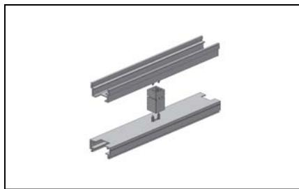
*Figure above showing center baluster attachment
