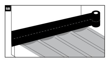
»Fold the Trex Seal Ledger Tape in half. Remove one of the release liners. Press to seal against the vertical surface at the 5-1/2" line. (5C)
