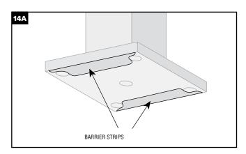
»Insert the (2) stainless steel barrier strips under the mounting bolt holes. Barrier strips are required only if attaching post directly to pressure treated framing.
