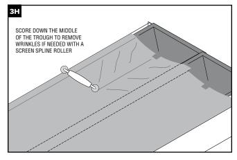
NOTE: In extreme temperature swings, trough material will expand and contract. Some wrinkling is acceptable but should not impede the flow of water.
