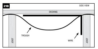
»Cut hole to fish wire going up through side of joists. Apply butyl caulk around wire and tape over wire and caulk. (21C)
