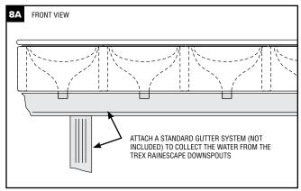
NOTE: Installing a clean-out trim piece will allow access to gutter line after installation.
