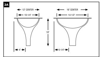
»Downspout should extend 1" into gutter: cut or extend as necessary. (2C)
