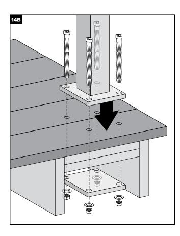
»Attach posts using four 3/8" x 6" (1 cm x 15.2 cm) hex cap bolts, washers, and nuts, along with aluminum back plate on underside of blocking.
