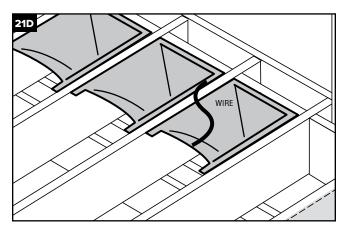
»Fish wire up through the gap between the trough and downspout. (21D)
