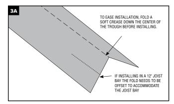
»When working with the Trex RainEscape trough material, ensure that the smooth/shiny side always faces up.
