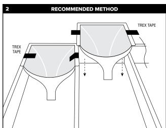
»Take 3-4" strips of our Trex butyl tape to hold downspouts to deck joists. Tape on either side of downspout to secure.
