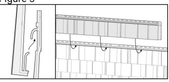
5-RoughSawn corners must be installed on wall corners prior to installing the RoughSawn Single sections. See the corner installation section as needed.
