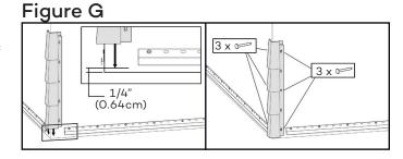
3-After installing some rows of product until one row overlaps the upper corner. Adjustments may need to be made at the vertical overlap of the two corners (as they are installed) in order to maintain the proper corner/section alignment. There is approximately a 1/2"(1.27cm) vertical adjustment value. To do so, only remove the fasteners at the center holes of the upper corner. Adjust its position and put the fasteners back into the center holes of the corner.
