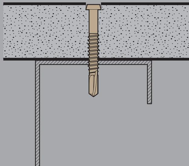
Note: Wings on 1 5/8" Deckfast Metal are designed to shear off during installation.
