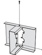
The 10 x 1 5/8" version of Deckfast Metal is designed for decking materials with an actual thickness of 3/4" to 1" attached to steel or aluminum up to 12 gauge or two 14 gauge joists doubled up. The 12 x 2 3/8" version of Deckfast Metal is designed for decking materials with an actual thickness of 1" to 1 1/2" attached to steel or aluminum up to 3/4" thick. Both versions are Trex® approved.
