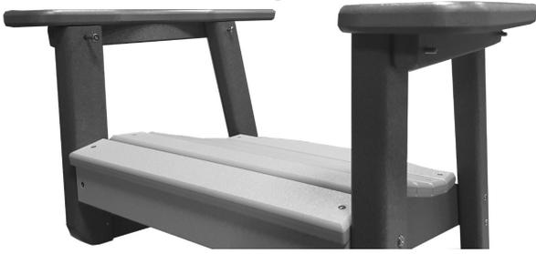
3. Attach the arms using four 3" bolts. The bolts go from the inside of the arm supports out through the arm. Place a flat washer, lock washer and nut onto each bolt and hand tighten only.
