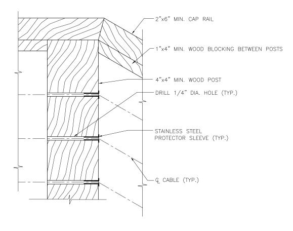
NOTE: INSERT PROTECTOR SLEEVES IN ALL HOLES WHERE CABLE ENTERS AT AN ANGLE TO PREVENT THE CABLE FROM CUTTING INTO THE WOOD. (I.E. STAIR TRANSITION POSTS OR OUTSIDE FACES OF DOUBLE CORNER POSTS)
