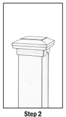
Fasten post cap to the post using 2 each provided screws or silicone adhesive.
