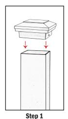
Test fit post cap to post to ensure that the cap is the proper size for the post.
