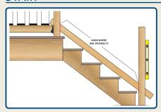
**STEP #1** - Lay bottom rail alongside posts and mark for angle. If posts are plumb top rail should be the same length and angle. Cut top and bottom stair rails at proper angle.
