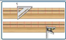
STEP #3 - Lay top and bottom rails beside each other and flush ends. Find the center of rails and mark lightly. Measure out 4-1/2" from both sides of center line and mark lightly. End spacing will vary. Set a combination square for center (example: 1-1/2" = 3/4") and mark lightly. Where lines intersect will be the center of baluster.
