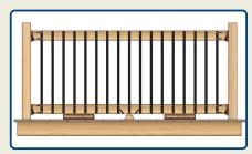
STEP #6 - Rest rail section on two (2) temporary spacer blocks the required height between deck and bottom of bottom rail. Center railing connectors on post and install four (4) #8 x 2" screws (per connector) through railing connector into posts. NOTE: With spans greater than 6' (or required), install a foot block (use cut-off from rail).
