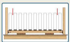
**STEP #5** - Cut two (2) temporary spacer blocks the required distance between deck and bottom of rail. Rest bottom rail on spacer blocks and center on mounting surface. Install four (4) #8 x 2" screws (per connector) through railing connectors into posts. Apply a small amount of silicone caulk to inside of glass baluster connector shoe to insure a tight, movement-free installation. Insert glass balusters into glass baluster connector shoes.
