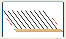
**STEP #4** - Make sure connectors are properly lined up. Apply a small amount of silicone caulk to diameter of baluster where it meets baluster connector or insertion hole to insure a tight, movement-free installation. Install balusters on bottom rail.
