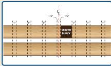
STEP #3 - Find center of top and bottom rails. From center line, measure and mark 1/2" on both sides of center mark (marking a 1" space). Cut a 3-1/2" spacer block and hold against the outside edge of center 1" space. Repeat process on other side of center and continue across rail. NOTE: 3-1/2" is a "Starting Point" it may be necessary to adjust spacing depending on rail length. Do not exceed 4" gap between balusters.
