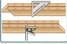
**STEP #2** - Lay top and bottom rails beside each other with the top rail turned upside down. Position rails as shown. Find the center of rails and mark **lightly**. Measure out 5-1/2" from both sides of center line and mark **lightly**. End spacing will vary. Set a combination square for center (example: 1-1/2" = 3/4") and mark **lightly**. Where lines intersect will be center of screw/insertion hole.
