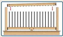
**STEP #6** - Start Top Rail at an angle and insert connectors into balusters or balusters into insertion holes in top rail. Make sure balusters are fully connected. Install four (4) #8 x 2" screws (per connector) through railing connectors into posts.
