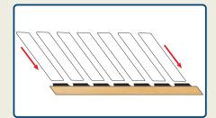
**STEP #4** - Apply a small amount of silicone caulk to inside of glass baluster connector shoe to insure a tight, movement-free installation. Insert balusters in bottom rail connector shoes.
