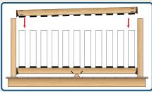
**STEP #6** - Start top rail at an angle and insert balusters into glass baluster connector shoes. Install four (4) #8 x 2" screws (per connector) through railing connectors into posts. NOTE: With spans greater than 6' (or required), install a foot block (use cut-off from rail).
