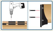
STEP #4 - With 8" center marks measure over 2-1/2" (this will be the edge of glass baluster connector shoe). Center baluster shoe on rail and insert screws though connector shoe. Make sure screw head is inserted below Glass Baluster.
