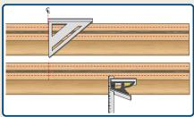
STEP #3 - Lay top and bottom rails beside each other and flush ends. Find the center of rails and mark lightly. From the center mark, measure out 8", from both sides and mark. End spacing will vary. Note: Baluster spacing will vary with rail length
