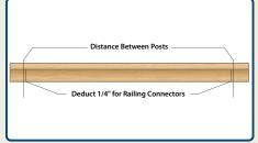
STEP #2 - Using step - 1 measurement, deduct 1/2" from total measurement for railing connectors. Cut both top and bottom rails.
