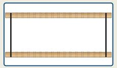
STEP #4 - Lay rails on a flat surface & install the two (2) outer balusters (four (4) screws per baluster). This will maintain spacing between rails.
