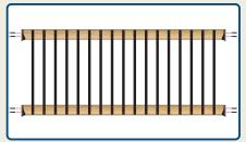
STEP #5 - Finish installing balusters. Slide railing connectors on rail ends making sure rail is fully seated in connector. Install two (2) #8 x 2" screws (per connector) through railing connectors into rail ends.
