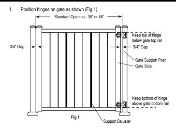
2. Follow installation instructions included with hinges and latches. *NOTE: Align gate rails with adjacent railing when attaching gate to gate support post.*
