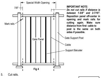
6. Cable(s) 1-5/8" or less from end of rail must be cut and removed from panel (Fig 5).
