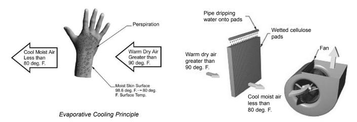
Evaporative cooling is the same process your body uses to cool itself. When you perspire, and air moves across your skin, a portion of the perspiration (water) evaporates. Evaporation requires heat to change liquid water to water vapor and this heat is taken from your skin, producing the cooling effect.
