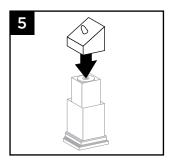
Follow all other instructions as stated above. Ensure that foot block is placed at location where hole was drilled in lower stair rail to allow for foot block to fit properly.
