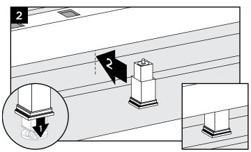
2. Slide foot block sleeve over foot block base. Position under bottom rail at location where hole was previously drilled.
