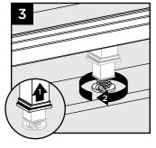
Mounting holes on turn mount should be facing out to allow for attachment to decking surface.
