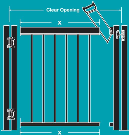
**Gate Assembly and installation;** gate are designed to fit an opening of up to 48" and the width may be cut to fit.
