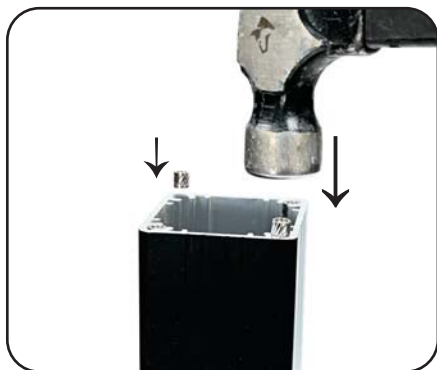
Adjustable Top Plate - Step 1 Tap Screw inserts down into the post screw bosses using a hammer until flush with the post.
