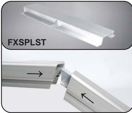
Series 200 - Stair Splice - Step 1 Splice slides into each end of the rail. Bend splice to the correct angle of the stairs and secure splice into place with 8 ea. screws.
