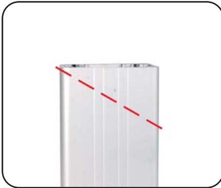
Series 200 Stair Posts Post must be cut at the angle of the stairs to allow for proper top rail attachment.
