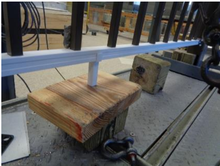
Photo No. 20 Outlook Series - Bottom Rail Support Block
