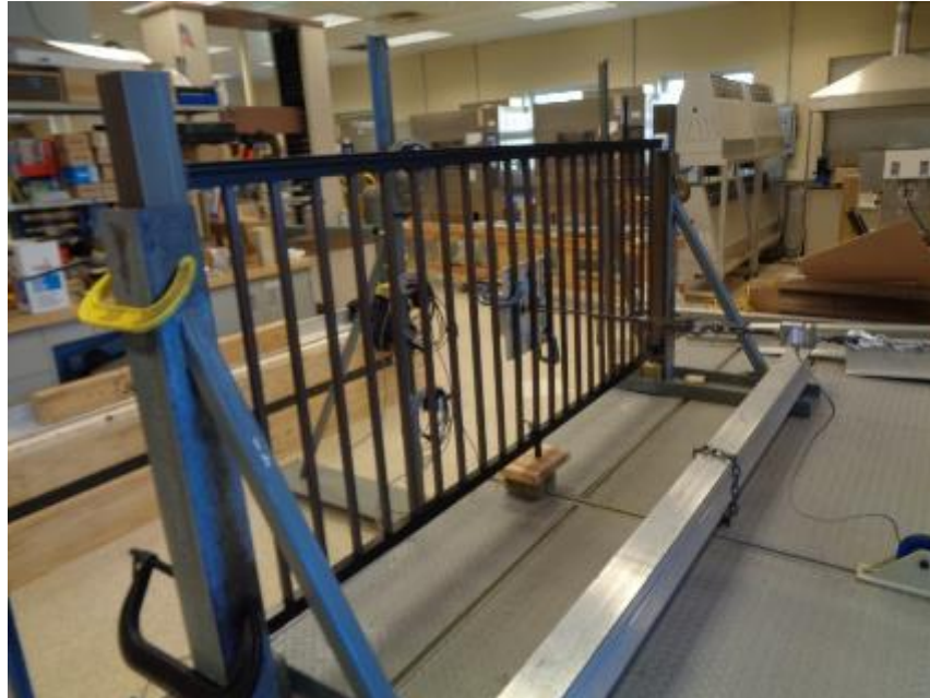
Photo No. 5 In-Fill Load Test at Center of Two Pickets
