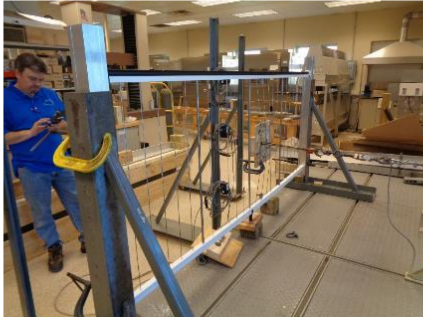
Photo No. 3 In-Fill Load Test at Center of Vertical Cable Infill
