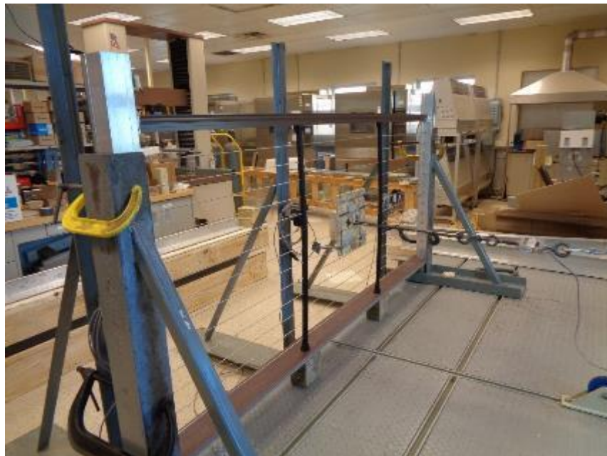
Photo No. 2 In-Fill Load Test at Center of Horizontal Cable Infill
