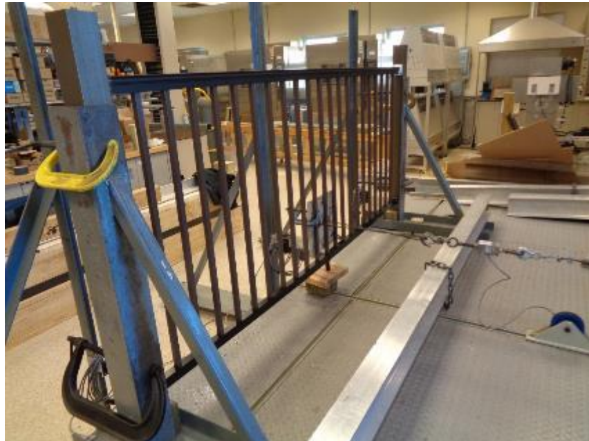
Photo No. 7 In-Fill Load Test at Bottom of Two Pickets
