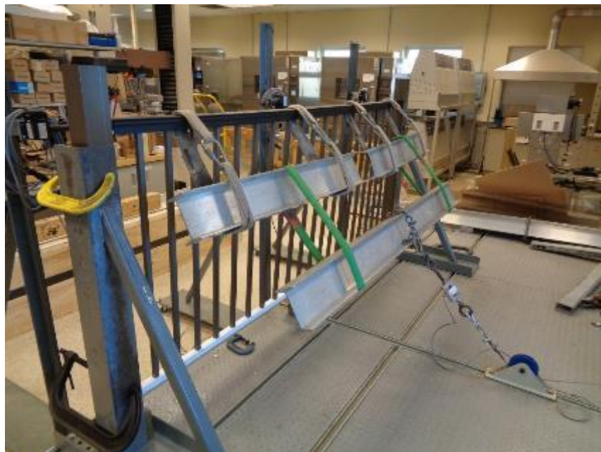
Photo No. 8 Uniform Load Test on Top Rail
