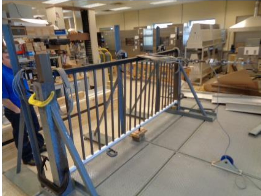
Photo No. 9 Concentrated Load Test at Mid-Span of Top Rail
