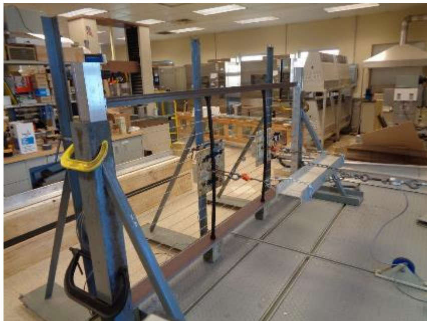
Photo No. 4 In-Fill Load Test at Center of Intermediate Support Balusters
