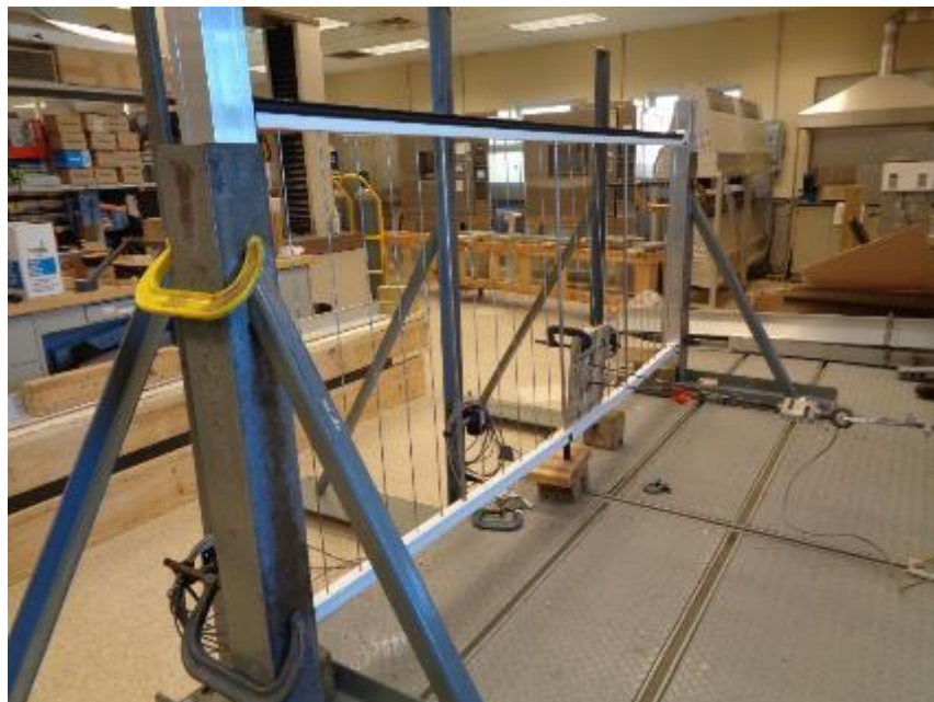
Photo No. 6 In-Fill Load Test at Bottom of Vertical Cable Infill
