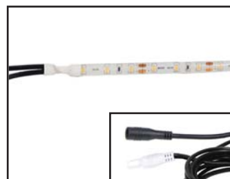
30" Strip Light 2.5 Watt 2 - Leads per fixture 1 - 12" Lead (Black) 1 - 6' Lead (White)
