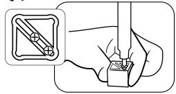
Align plug in center of bottom of the bottom rail. Be sure aluminum is centered in rail prior to securing plug to rail.
