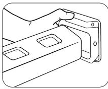
Place rail brackets on ends of bottom rail.
