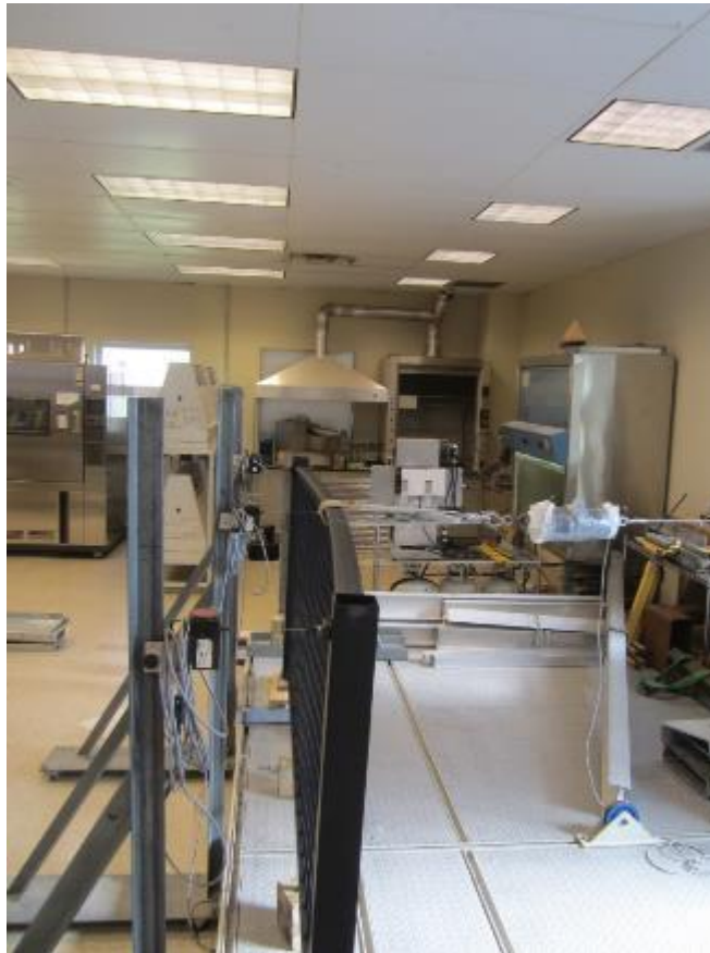
Photo No. 6 Concentrated Load Test at Mid-Span of Top Rail
