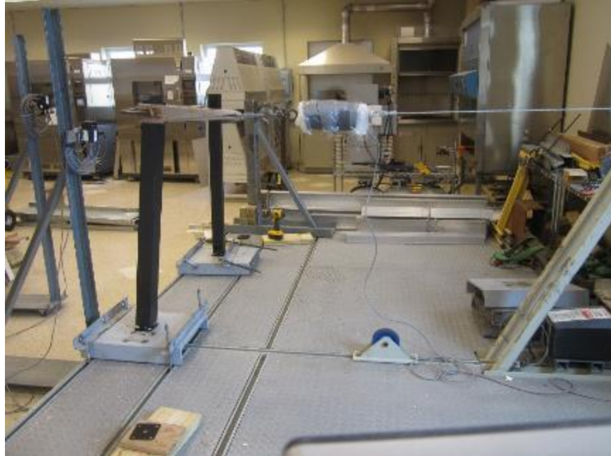
Photo No. 9 Concentrated Load Test at Top of Post Mount (Simulated Concrete Installation)
