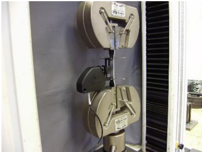
Photo No. 2 Typical ASTM E 8 Tensile Test Setup
