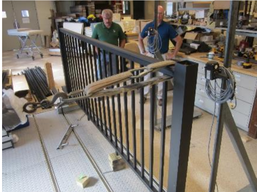
Photo No. 7 Concentrated Load Test at Rail End (Bracket)
