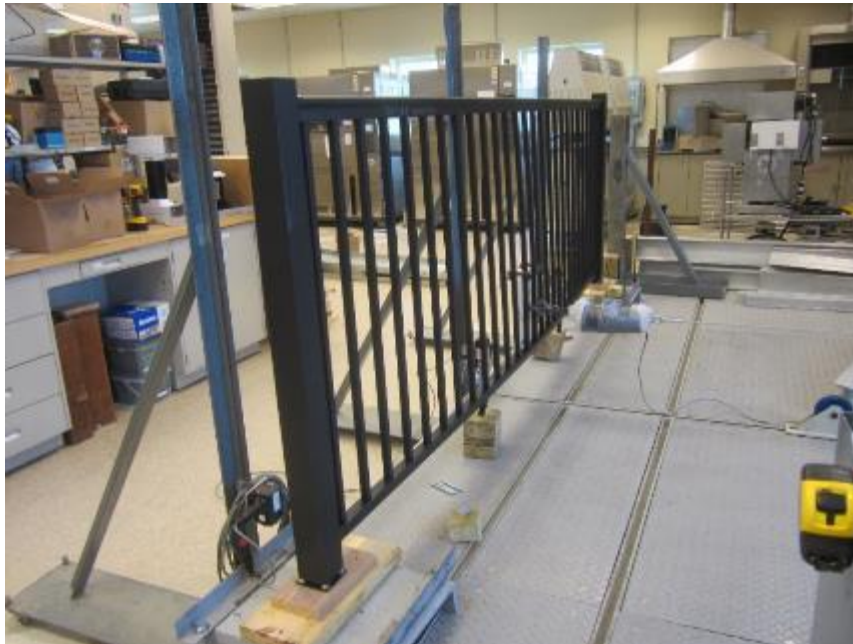
Photo No. 5 In-Fill Load Test at Bottom of Two Pickets
