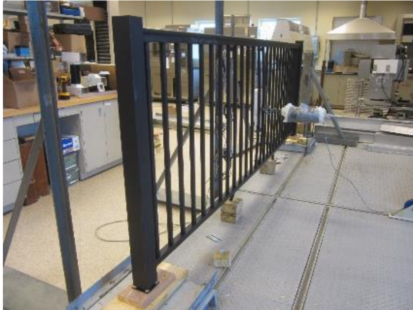
Photo No. 4 In-Fill Load Test at Center of Two Pickets
