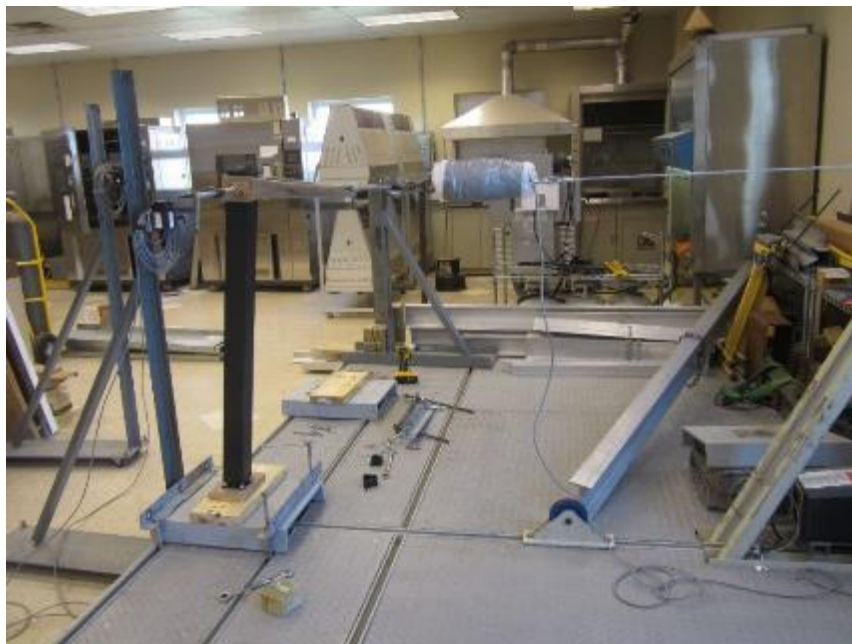
Photo No. 8 Concentrated Load Test at Top of Post Mount (Surface Mount Wood Installation)
