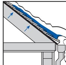
Grace Ice & Water Shield® underlayment resists this leakage because of the seal around the fasteners, ability to make water-tight laps, and the membrane's bond to the deck.
