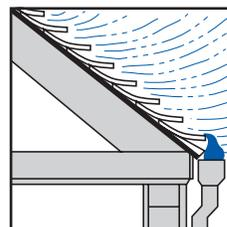
Grace Ice & Water Shield® roofing underlayment applied beneath the sloped roof covering helps prevent wind-driven rain from entering the structure.
