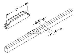
Cut Rails to required length. Place top and bottom 2x4 rails side by side for accurate placement of Fortress Pure View Nylon Mounting Shoes. Fortress Pure View Glass Balusters CANNOT EXCEED 4" SPACING between balusters. Mark layout on rails so that there is a equal distance between the first Pure View Baluster and the end of rail at each end. Using a square mark the location of each Pure View Nylon Mounting Shoe and pre-drill with a 1/16" drill bit.
